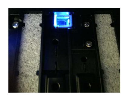
Actual CMOS sensor photographs the back-side of the media in realtime to help determine media movement.
