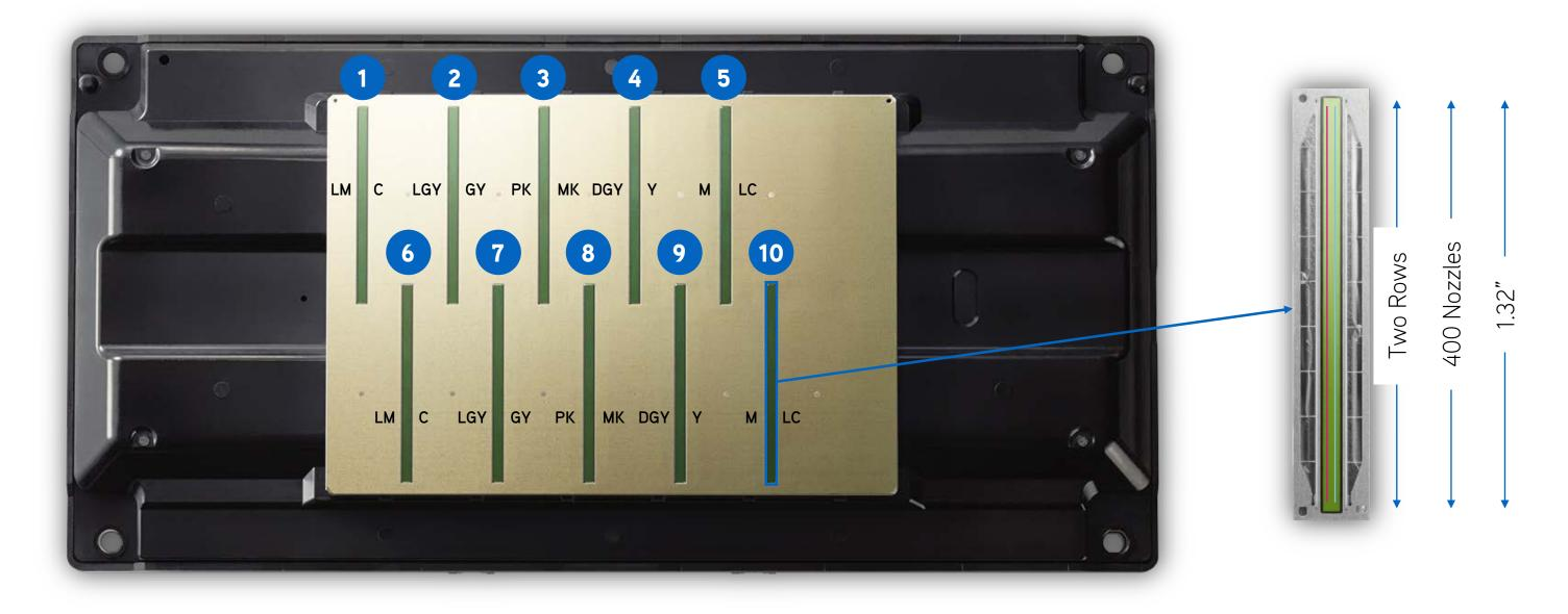
The PrecisionCore MicroTFP printhead is developed using 10 individual PrecisionCore "blades". Each "blade" has two rows - one for each color - using 400 nozzles each across a 1.32" width. When combined, the final printhead array prints using 800 nozzles per color over a 2.64" print width.
