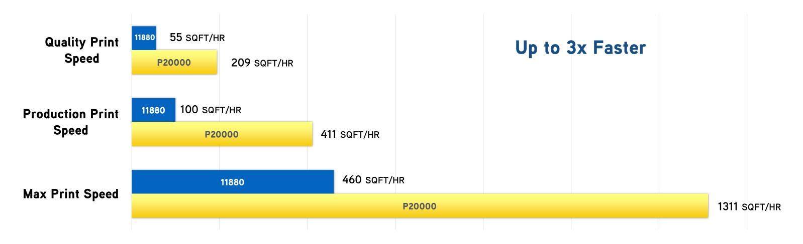
Print times are based upon start of printhead movement over the page to drop ink - Stop time based on printhead moving to park position
